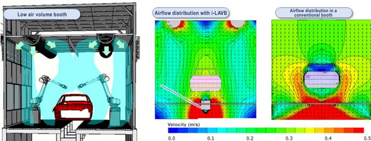
Our i-LAVB proposal redesigns the conventional paint booth full-surface air supply structure, allowing air to be supplied to areas where it is needed, such as the painted body or around the booth walls. By optimizing the airflow in the paint booth, the air supply air volume required to maintain the paint environment is greatly reduced. The introduction of the system reduces the energy needed for air conditioning as well as CO<sub>2</sub> emissions, helping contribute to carbon neutrality.
