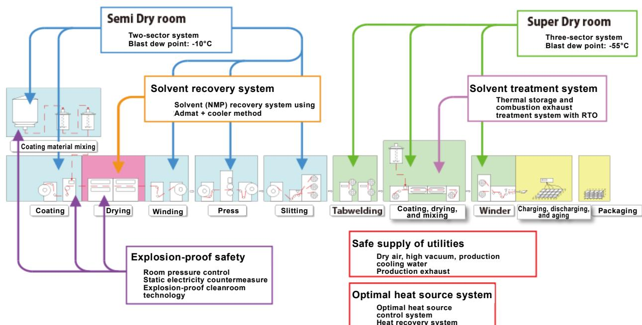
We provide low-cost, space-saving, high-performance dry rooms (low-dew-point manufacturing rooms) as a combined solution for air conditioning and exhaust treatment. Our revolutionary NMP Recovery System, in particular, boasts superior ease of maintenance, high energy savings, and low running costs, making it one of the best in Japan.
