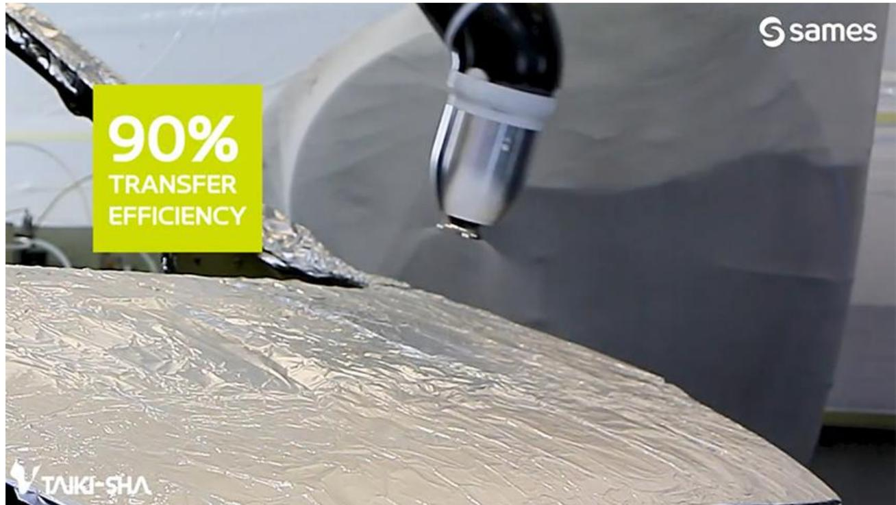
High paint application efficiency reduces wasted paint and VOC emissions. Minimizing paint splatter reduces the required ventilation air velocity, which also reduces the energy used. This also reduces the work involved in cleaning and reduces health risks.
