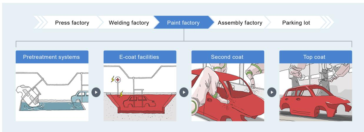
We will introduce energy-saving and environmentally friendly coating equipment technologies carefully selected from a range of proven technologies that have been introduced at numerous automotive plants.
