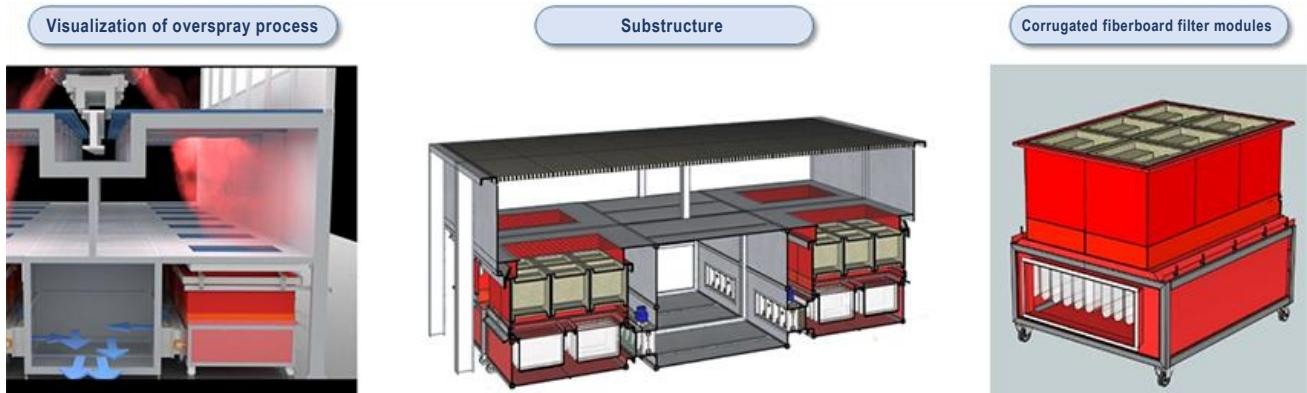
Our proposed i-Dry Scrubber is a dry paint booth that reduces overspray adhesion dust by means of a dry filter (corrugated fiberboard filter). Unlike conventional wet booths, no water is used to catch overspray, making it a powerful tool in areas where water is scarce.
