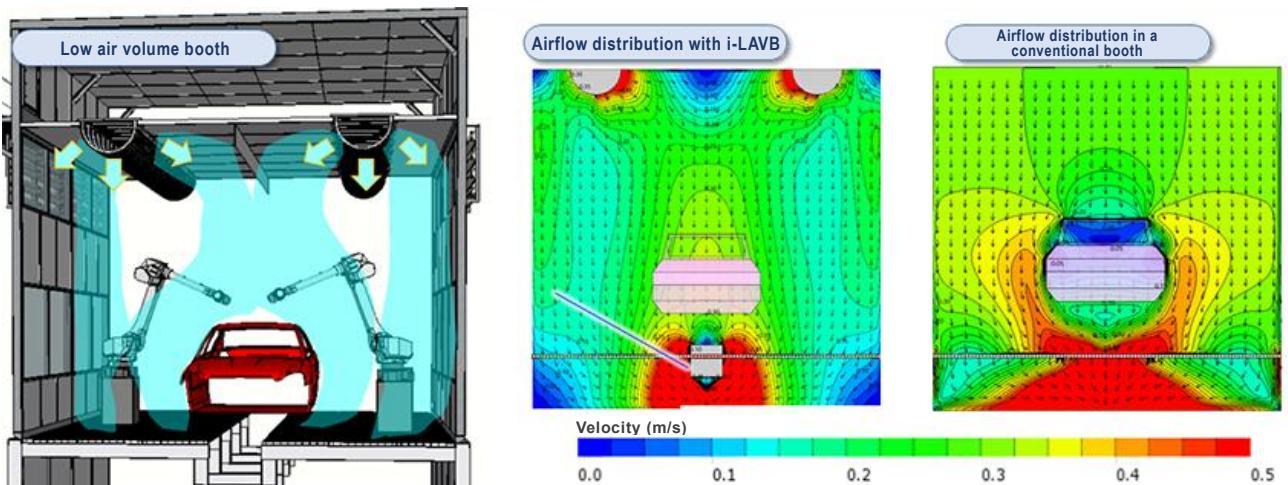
Our i-LAVB proposal redesigns the conventional paint booth full-surface air supply structure, allowing air to be supplied to areas where it is needed, such as the painted body or around the booth walls. By optimizing the airflow in the paint booth, the air supply air volume required to maintain the paint environment is greatly reduced. The introduction of the system reduces the energy needed for air conditioning as well as CO<sub>2</sub> emissions, helping contribute to carbon neutrality.
