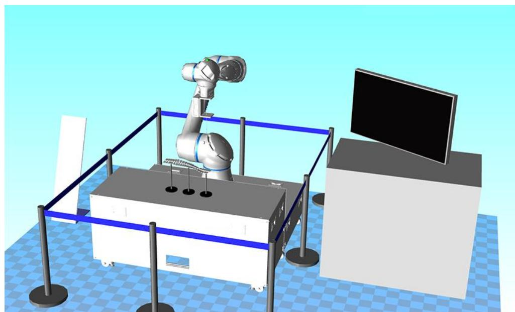
The system determines the shape of a workpiece and the target area, and creates robot motions from scratch with high accuracy, rather than correcting the position of the captured image.
